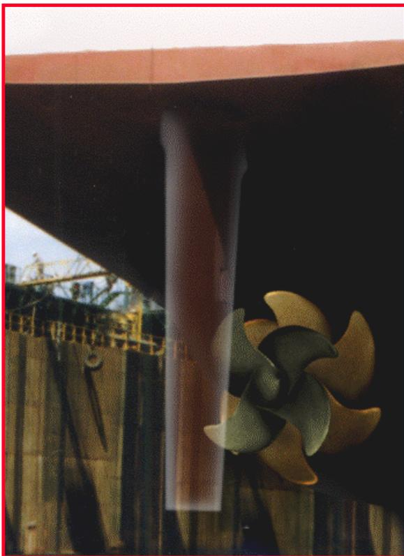
Figure 12 - Contra-Rotating Propellers
