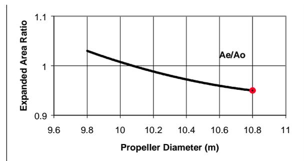
Figure 11 - Effect of Propeller Diameter on Required Blade Area Ratio (12,500TEU design)
