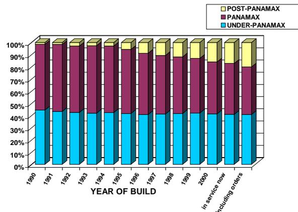
Figure 1 – Evolution of container ship fleet
