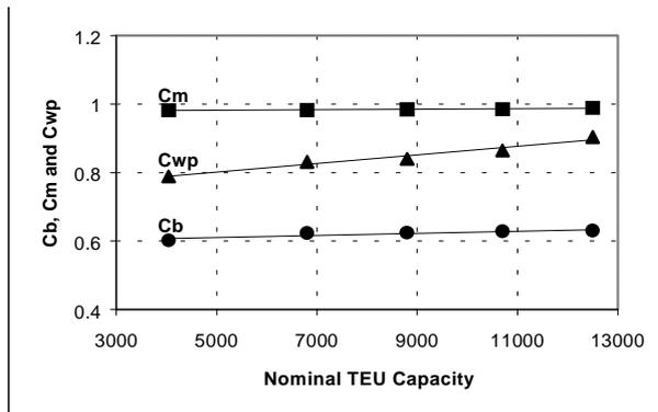
Figure 8 - Hull Form Coefficients
