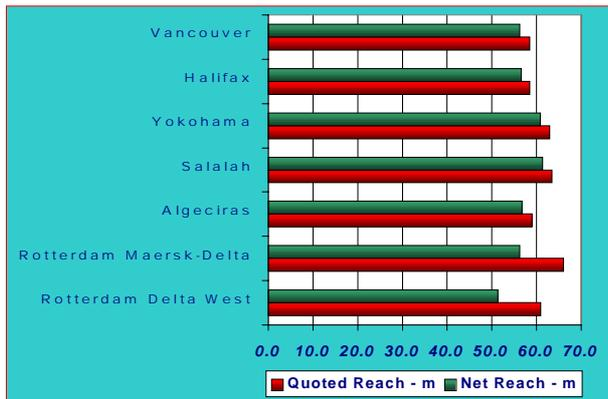
Figure 15 - Effective Crane Outreach at Potential ULCS Terminals
