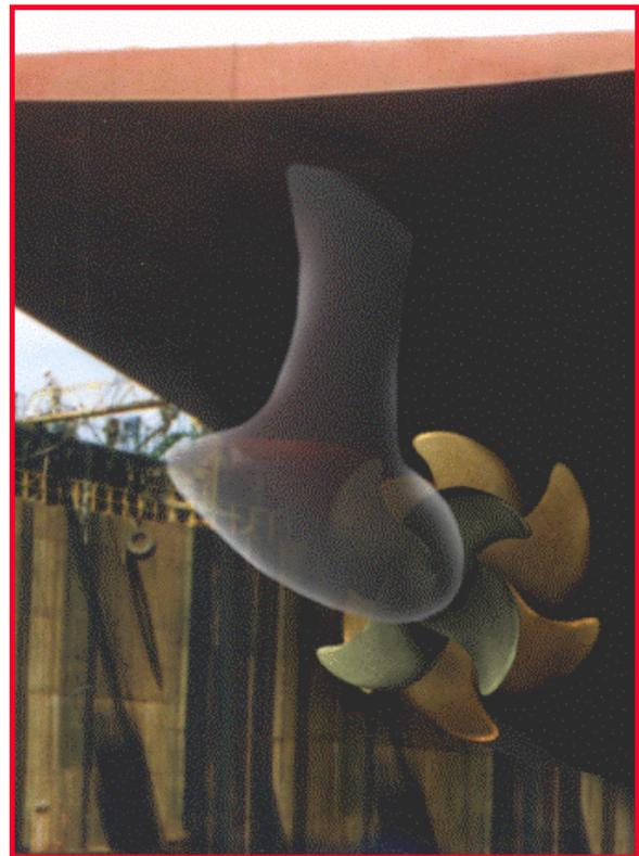
Figure 13 - Contra-Rotation using Podded Drive
