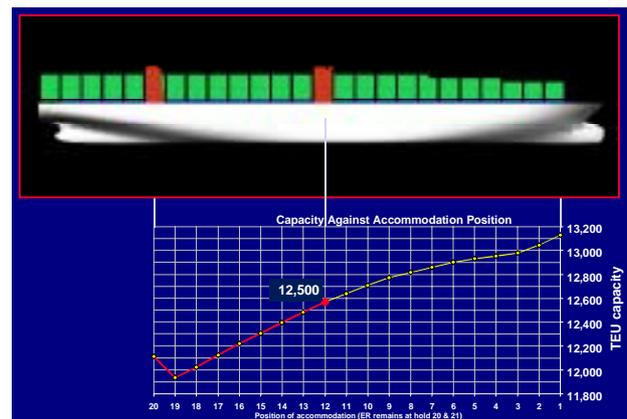
Figure 4 - Effect of Re-locating Superstructure
